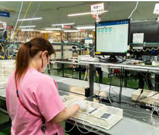
Diagnostic work at the processing center in Iwakura, Aichi Prefecture. Staff connect handsets to a PC with Blancco Mobile Diagnostics & Erasure installed.
